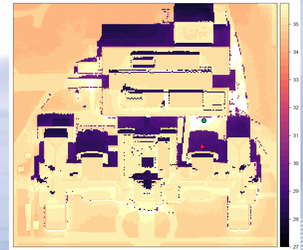
Fig. 7: As Fig. 6 but for the Universal Thermal Climate Index (UTCI). The two points (Sun and shade) inside Fig. 6 and 7 mark the position of the calculated outputs from Fig. 5 and 8.
